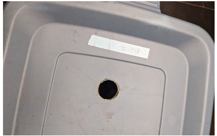
Figure 7. Top view of 18-gallon BSF larval rearing bin showing 1-inch circular opening for Tee PVC joint insertion. (Photo Credit: Catherine Terrell)
