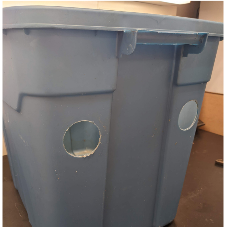
Figure 8. Side view of 18-gallon larval rearing bin showing 1-inch circular openings for PVC pipe to exit rearing bin. (Photo Credit: Catherine Terrell)
