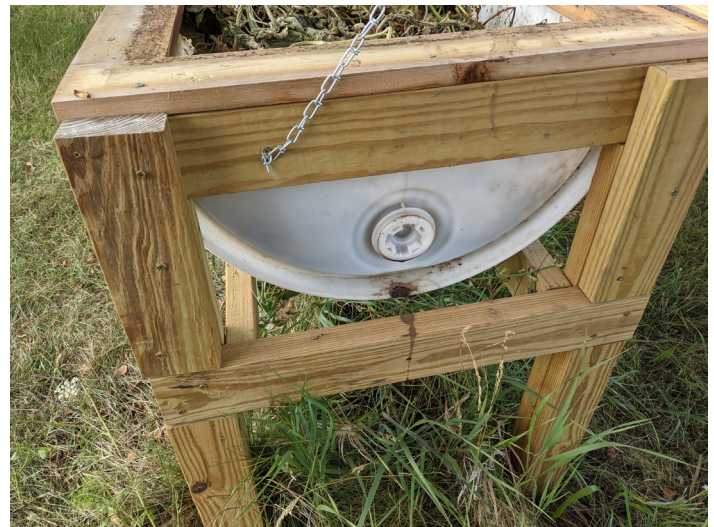
Figure 23. Inside of bin, mounted to legs and lined with 1x4 cut lumber. (Photo Credit: Catherine Terrell)
