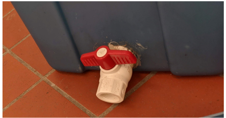
Figure 16. Drain valve that has been secured to rearing bin with caulk. (Photo Credit: Catherine Terrell)
