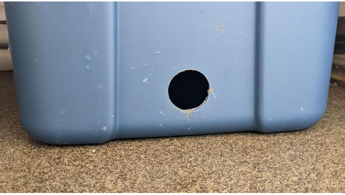
Figure 9. Drill hole for drain (optional). (Photo Credit: Catherine Terrell)
