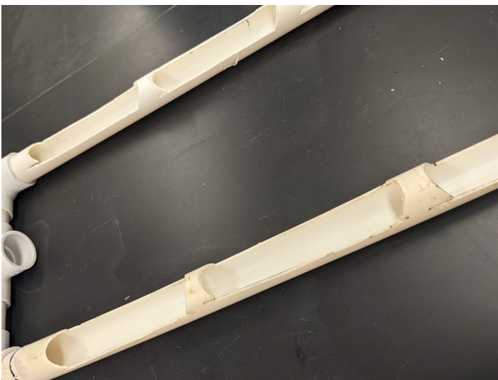
Figure 11. Smoothed edges of BSFL ramp targeted to fit into the bin around 35° to facilitate pupation outside of the bin. (Photo Credit: Catherine Terrell)
