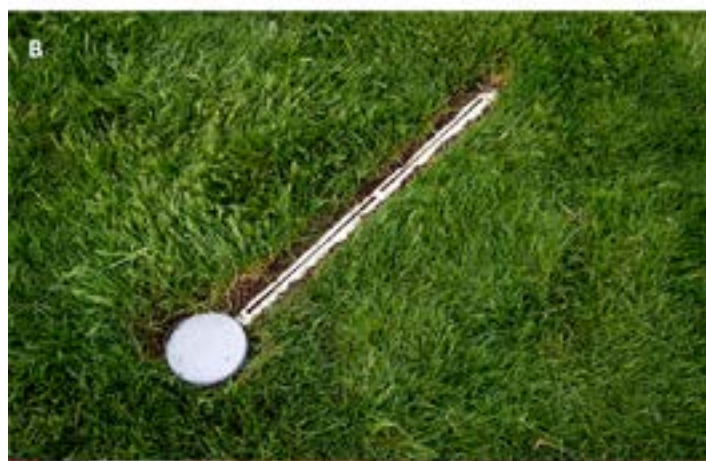
Figure 12. Plans for constructing a linear pitfall trap used to monitor adult billbug activity (A). Installed trap (B).
