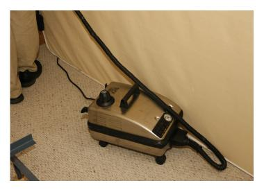
Steam equipment can be used to kill bed bugs. Vacuum machines can also be used to physically remove bed bugs. (*Photo credit: Tom Myers*)
