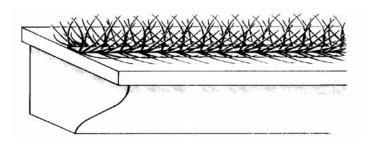
Figure 1. Porcupine wires can be used on various building surfaces to prevent pigeons from roosting.
