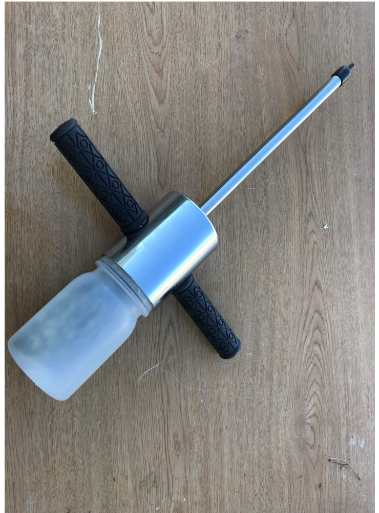
Use of a hay probe results in more accurate forage quality data as compared to sample collection by hand.
