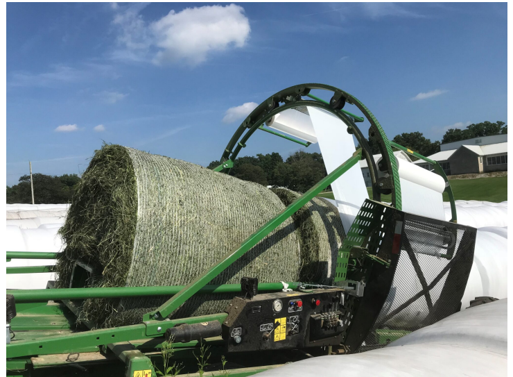
An in-line bale wrapper applies ultraviolet-light resistant plastic wrap to round bales so fermentation can occur. (Photo Credit: Keith Johnson)
