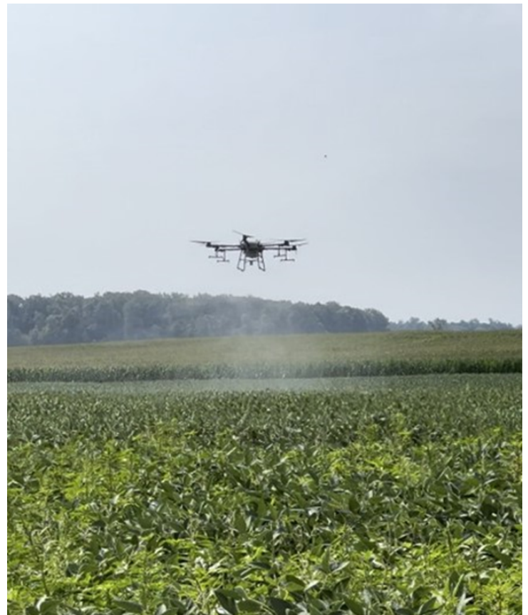
DJI T30 UAS with the payload capacity of 7.9 gallons. Photo Credit: M. Mizuno, Purdue University.
