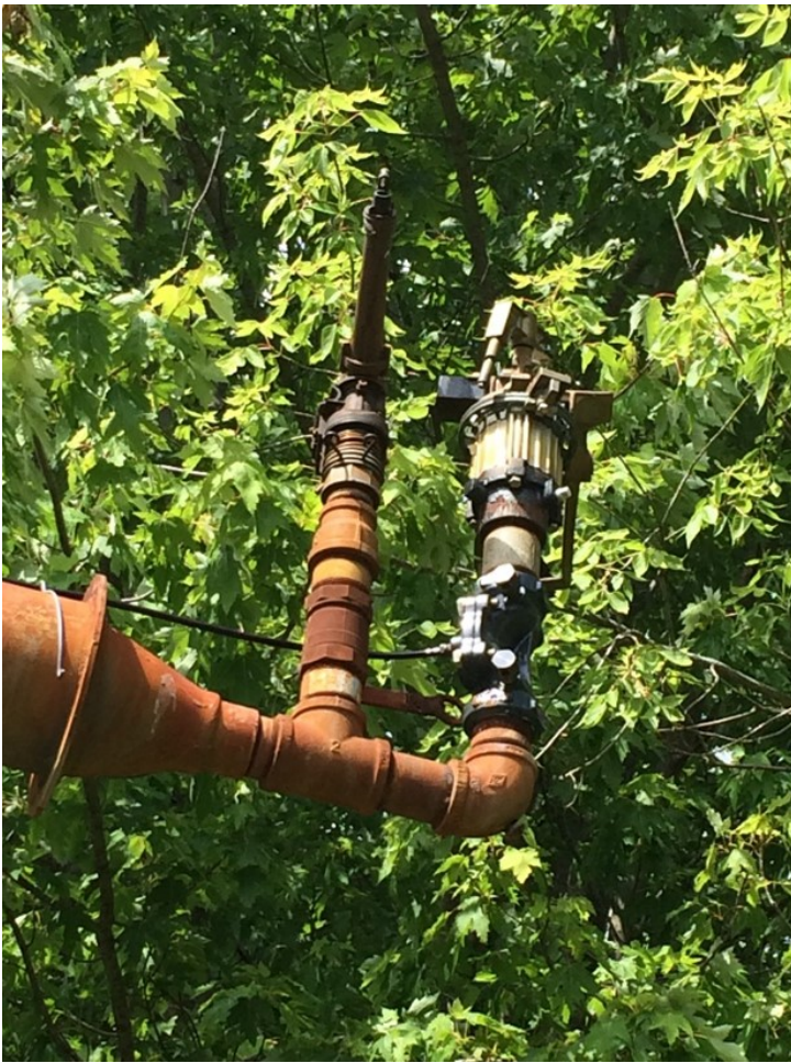
Unchecked fence row tree and brush growth into the path of the end gun and pivot end boom can create major damage. Photo by Lyndon Kelley, MSU Extension.
