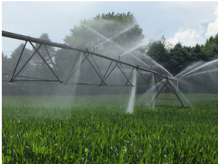
It is rare to find this many leaks in one place, but worn-out pipe flange gaskets, rust holes in the bottom of the pipe, and supply line leaks are common challenges. Photo by Lyndon Kelley, MSU Extension.
