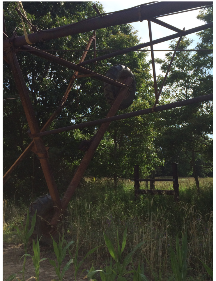
The stop barricade normally contacts the electronic stop arm, turning or reversing the system. The stop should not allow the wheel to climb resulting in rollover of the last span. Photo by Lyndon Kelley, MSU Extension.
