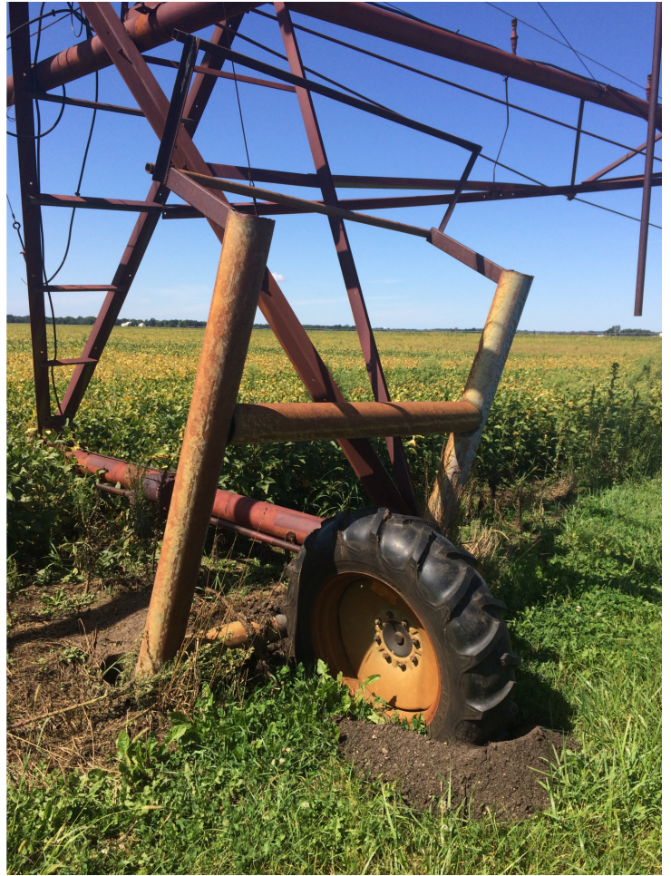
Stop barricade design and construction should stop the forward movement of the tower and cause the drive tire to slip and not climb the stop barricade. An electronic control in the next to the last tower (over watering timer) will cause the pivot's safety system to shut the system down after the tower has not moved for a few minutes. Photo by Lyndon Kelley, MSU Extension.
