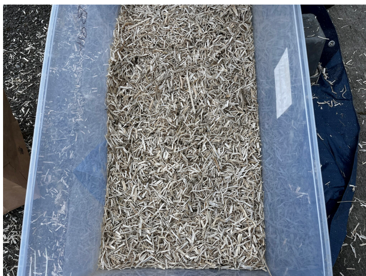
Fig 3. Hemp hurd is the inner pithy component of the stalk.
