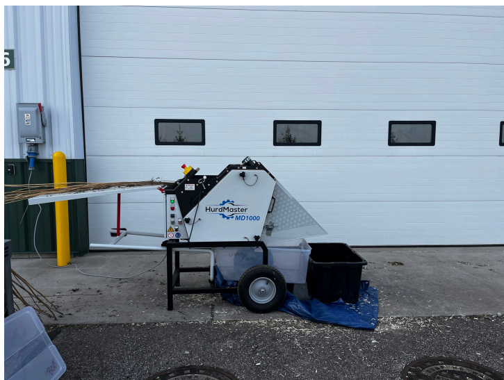
Fig 1. The HurdMaster decorticator is used for processing whole hemp stalks out at the ICSIC.
