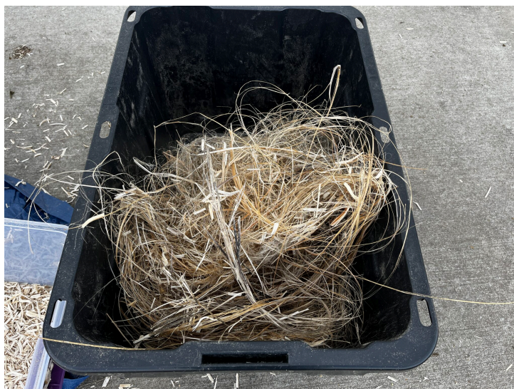
Fig 2. Hemp bast is the outer long fibers of the stalk.
