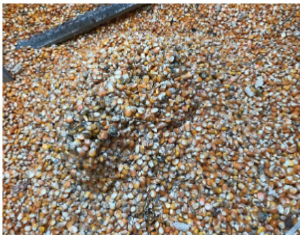
Figure 2. Hotspot development observed from the surface of grain in a bin.
