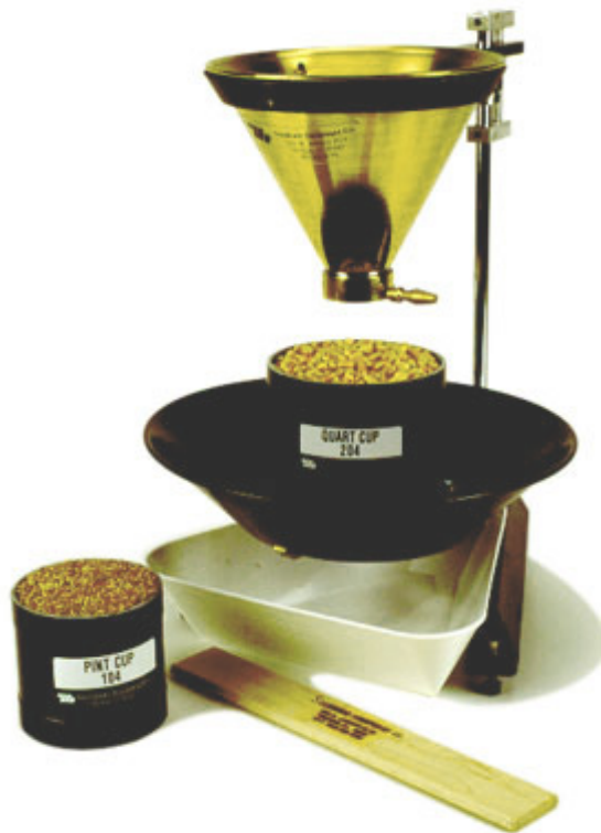
Fig. 1. A standard filling hopper and stand for the accurate filling of quart or pint cups for grain test weight determination. (Image: www.seedburo.com).
