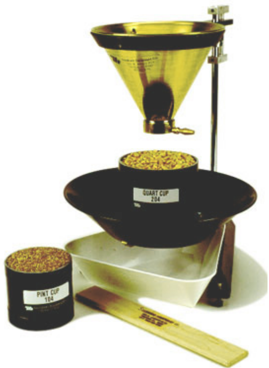
Fig. 1. A standard filling hopper and stand for the accurate filling of quart or pint cups for grain test weight determination. (Image: www.seedburo.com).
