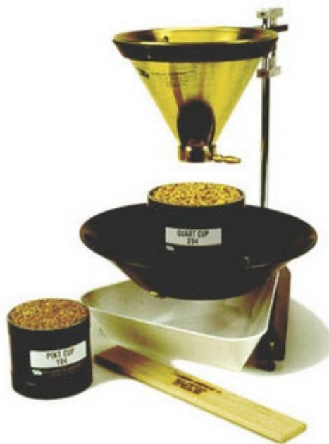
Fig. 1. A standard filling hopper and stand for the accurate filling of quart or pint cups for grain test weight determination. (Image: http://www.seedburo.com ).
