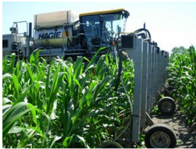
A solid shank applicator applying N to tall corn.
