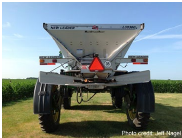
High-clearance box spreader spreading granular urea.
