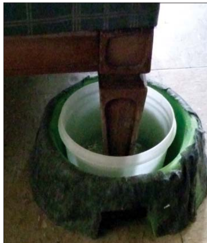
Figure 1: The experimental bed bug interceptor consisted of two plastic bowls. A small inner bowl (white) contained a mixture of diatomaceous earth (50 percent) and talcum powder (50 percent) as a killing agent. The large bowl (green) contained 40 ml 50 percent ethylene glycol as a killing agent.
